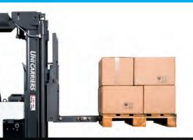
AJN/ASN and XJN/XSN have the possibility for the addition of the telescopic forks, therefore becoming ATF and XTF. These trucks allow doubledeep handling to reduce aisle widths even further, or even loading and unloading transport from just one side. In some applications, this function can replace a small reach truck.
