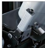
The light-touch parking brake lever has a safety device that keeps the lever from being released until the button on the end is pushed.
