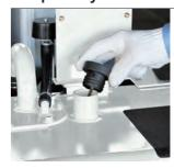
The hydraulic oil filler cap is a snap-fit type which allows easy removal and reinstallation. Attention to detail has been paid in order to assure better work efficiency.
