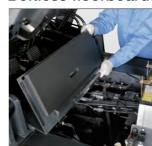
The boltless floorboards are easy to remove and reinstall, without having to use any tools, for better truck serviceability.
