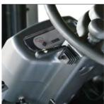
The automatic transmission is standard for smooth starts and acceleration, eliminating the chore of shifting gears. The electric directional control lever makes it easy to change the direction of travel.
