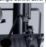
Single Control Lever allows for simultaneous lifting and tilting operations, for greater productivity.
